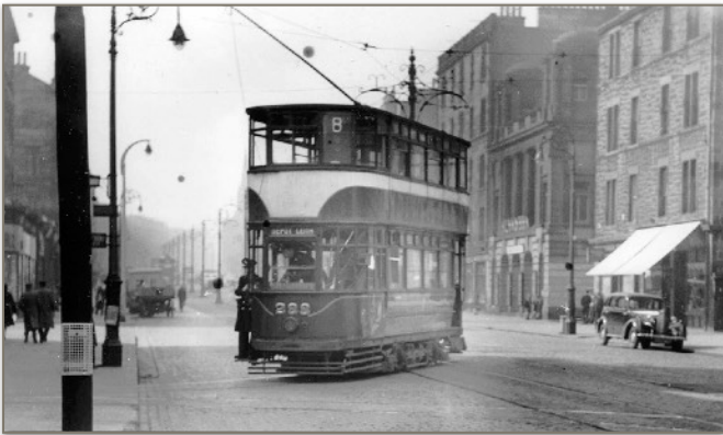
Pic 1: Wooden standard car 288 (built 1923 by Leeds Forge at Bristol) turning into Leith Depot with the conductor carefully holding the trolley rope guarding against any sudden de-wirement!
